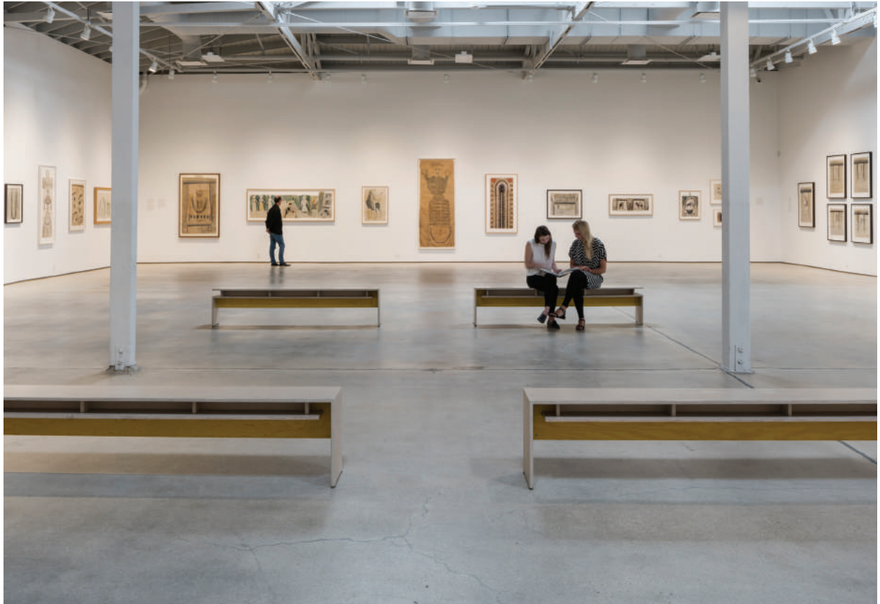
Ibid Gallery is formed from a bow-string trussed warehouse space, with new walls offset from the existing structure to frame the existing architecture and artworks. Photo: Jeff McLane.
